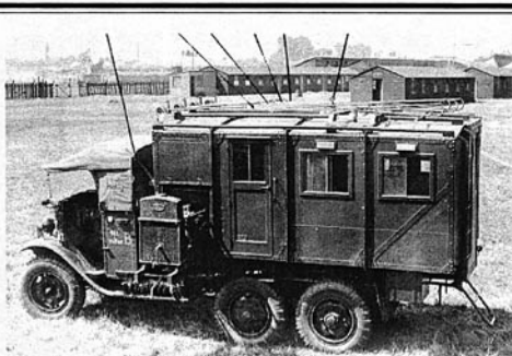
(Figure 2-7) No. 2 Set installed in a Morris 25-HP 6-wheeler with Aerial, Roof, No. 3. The generating set and accumulators are mounted in the forward compartment, accessible through the door of the fitter's compartment in the centre. The rear compartments of the vehicle body housed the operators and the No. 2 Set which was fitted to the partition wall
