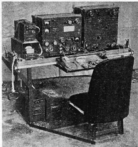
(Figure 2-8) Operating position of Wireless Set No. 2 removed from the vehicle to form a ground station
